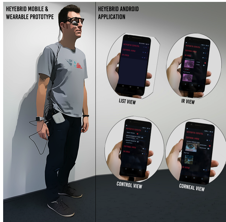
Fig. 1. The developed hEYEbrid concept used to build a mobile and wearable device for spontaneous competitive gaze estimation at any place and any time. The head-mounted device is connected to a Nexus 6P that processes both camera streams in real time.
