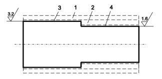
Fig. 1. Sample part cutting steps.
