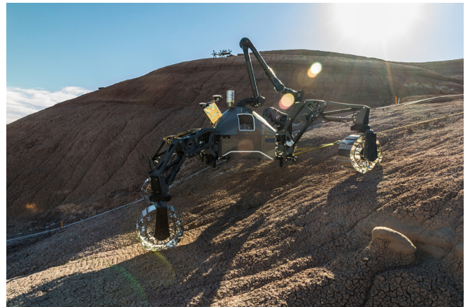
Fig. 1: The hybrid legged wheeled robot SherpaTT with a high amount of degrees of freedom and therefore high amount of magnetic field distortion sources during field trials in the desert of Utah, US
