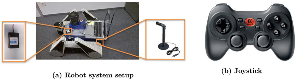
Figure 4.3: The robot setup for data collection showing where the sensors and laptop are mounted. Left side and right side of Figure 4.3a are the close up of the joystick receiver and Elecom Table microphone, respectively. While Figure 4.3b shows the logitech cordless rumblepad2 transmitter used for running robot manually.
