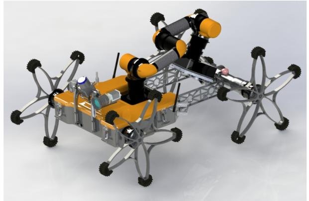
Figure 1. CAD model of Coyote III equipped with its manipulation device
