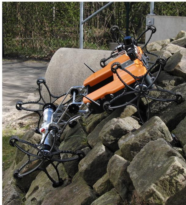
Figure 4. Coyote III in its current state, standing on a steep rocky slope
