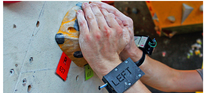
Figure 1. ClimbSense wearable sensors to automatically detect climbed routes with wrist-worn Inertia Measurement Units.
