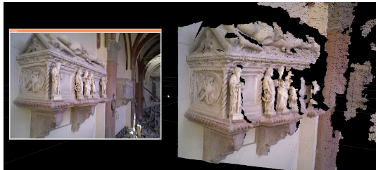
Fig. 6. 3D reconstruction of one of the Pico’s arks in San Francesco church, using data from the NIFTi UAV Kinect sensor.
