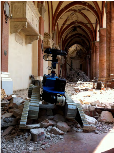
Fig. 4. NIFTi UGV with a rotating SICK-Laser (LMS100), a LadyBug3 omniscam, active flippers and active/passive bogeys, IMU, GPS, and a static mast mounting a PTU with a Kinect sensor.
