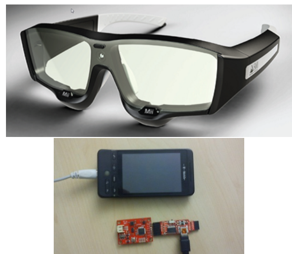
Figure 3. The new eye tracking device (top) and the sensor board (bottom). The board can be attached to the side of the eye tracker.
