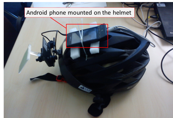
Figure 2. The Android phone mounted on the eye tracker helmet. the phone is tied up with a plastic cable and two cushions are put between the phone and the helmet.
