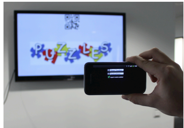
Figure 5: Device pairing. One possible way of pairing of the mobile device and the distant display by scanning a barcode on the display in order to send TUIO messages to the intended display.
