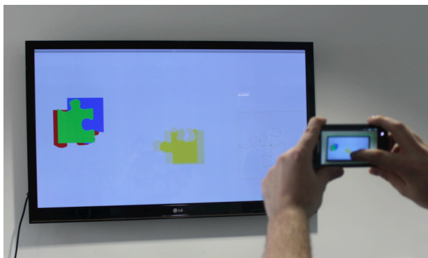
Figure 6: Example App. Puzzle Game. The user drags a puzzle tile by touching its representation in the live video on the mobile device.
