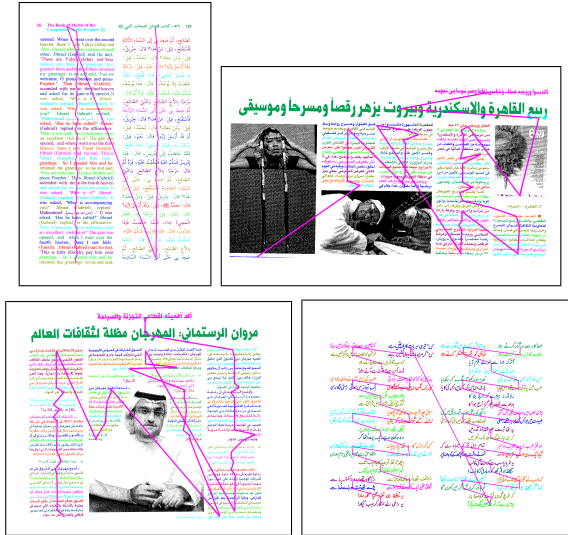
Figure 4. Sample images from Arabic and Urdu documents datasets and their corresponding layout analysis results: the black-pixels represents non-text components, the color coded labeling represent extracted text-lines and the magenta-line shows reading order of segmented text-lines. [top-left] Arabic-English book page; [top-right and bottom-left] Arabic newspapers (these images have been taken from the websites: http://www.alroostamanigroup.ae and http://www.mawred.org , respectively; [bottom-right] Urdu poetry image.
