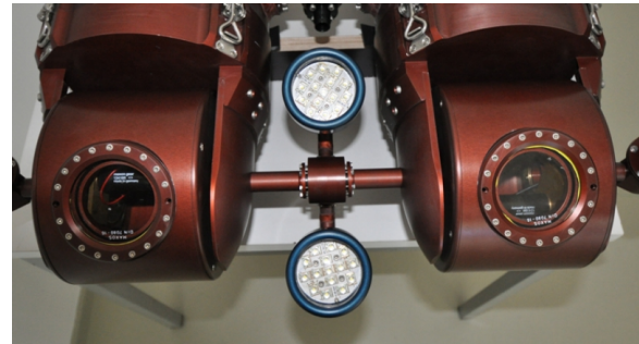
Fig. 5. Rotatable cameras with aligned LED light.
