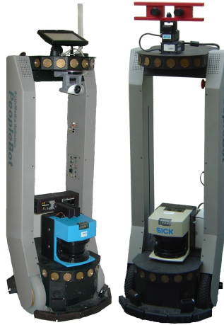
Fig. 10.3. The mobile platforms on which the Explorer scenario was developed and tested. Left: Minnie from KTH, Right: Robone from DFKI.
