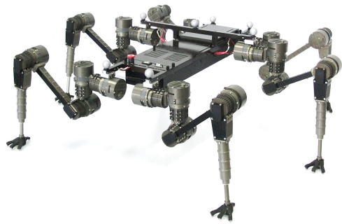
Figure 3. Integration study of the SpaceClimber robot. SpaceClimber is the antetype for the RIMRES scout system. A sensor head will be added for the prototype.
