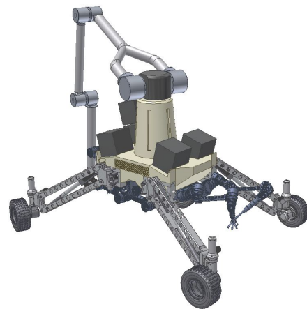
Figure 2. CAD-design study of the RIMRES rover. The rover provides four wheels mounted on an active/passive chassis system. Mounted beneath the rover in this CAD-drawing is the six legged scout robot. Shown on top are five payload modules (dark boxes).
