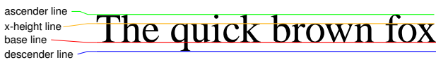
Figure 3: The anatomy of a text-line showing positions where characters align from top and bottom.
