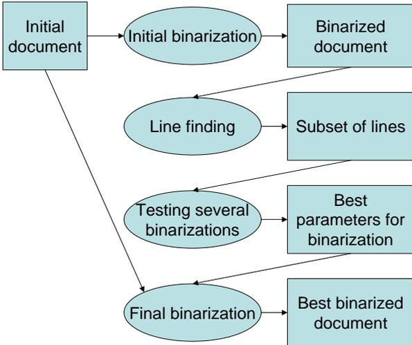
Figure 1: Recognition Driven Thresholding overview
