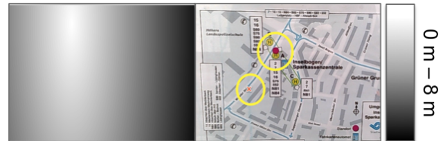
Figure 8: Mean error introduced by the “Two Point Referencing” approach. The error range (from 0m - 8m) was mapped on 255 grey-scale value (white pixel 0m error; black pixel 8m). The mean error was about 5m.
