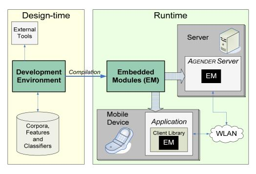
Figure 2. Architecture for device-based classification.
