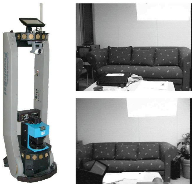
Fig. 5. The left image shows the robot used during the experiment. The right images depict examples for object detection: training couch image (top), detected couch image (bottom).
