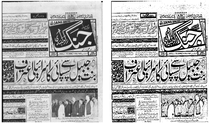
Fig. 6. An example image cropped from the front page of a newspaper containing both normal and inverted text in the same image. The binarization step fails to identify the inverted text and makes it a part of the page background (white) as shown in the binarized image.
