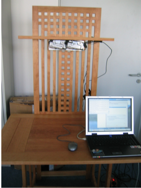
Figure 1. The complete setup: a wooden desk with two cameras attached and a laptop PC running the software components.
