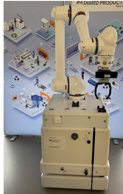
Fig. 3. Autonomous Mobile Robot for developing skills in intralogistics
