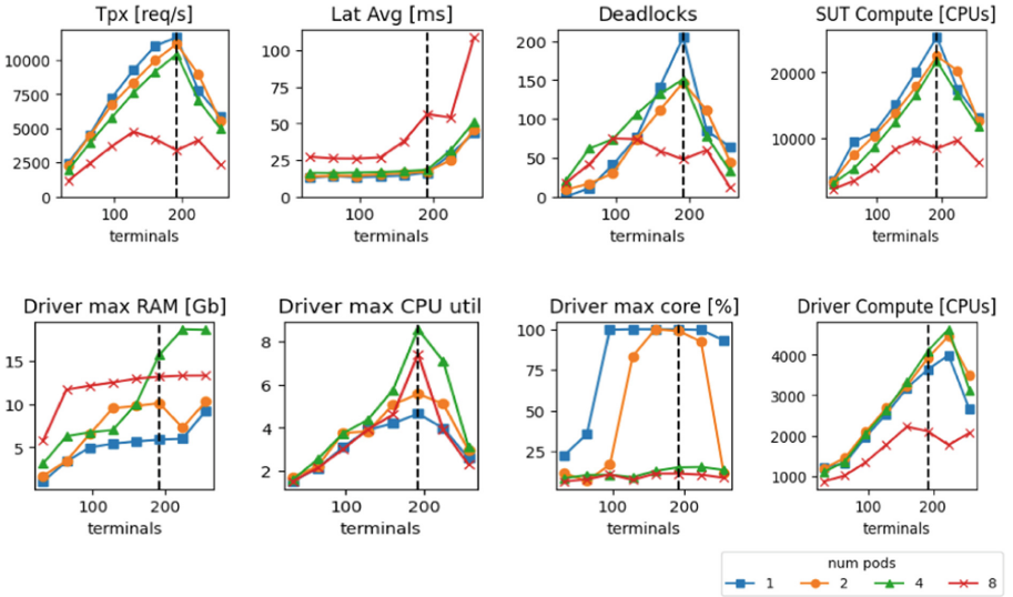
Fig. 10. Benchbase TPROC-C execution at 48 warehouses, target 16384 req/s
