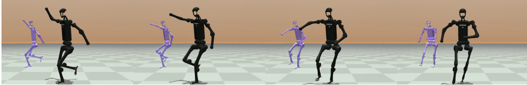
Figure 4: A latent space sequence for dancing is decoded by a reinforcement learning policy and executed in a physics simulator.
