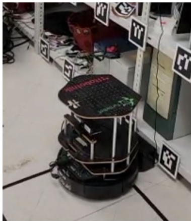
Fig. 16 Turtlebot2 (Kobuki) charging at dock station
