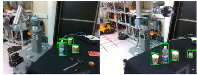
Fig. 9 Unknown object (left), rejected duplicate detection (right)
