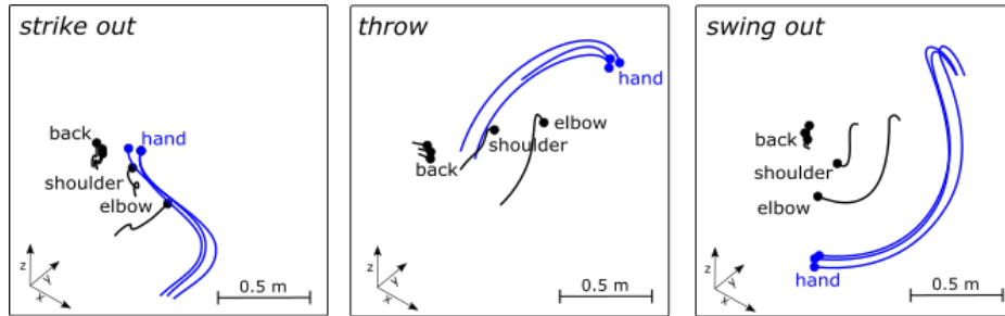
Figure 3.8.: Main throwing segments. Shown are the positions of the markers placed on back, right arm, and right hand. The lines show the movement, the end position of each marker is marked with a dot. The three hand markers are highlighted in blue.
