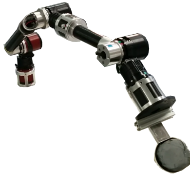
Figure 7.2.: Robotic arm COMPI with a spoon mounted as end effector. The ball that should be thrown was placed into the spoon. Image adapted from [Gutzeit et al., 2018a], Figure 3.
