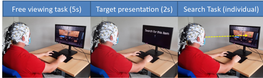
Fig. 1. Setup of the search task. The participant is shown the image on the left without a concrete target. Afterward (middle), the target is shown to the participant. The participant searches the target in the scene, and by gaze tracing, the object is highlighted and selected if the participant fixates on it for more than 2 seconds (right).
