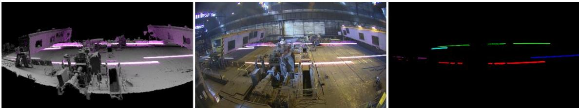
Figure 4 Left: A 3D model of the Saarstahl blooming train with inserted 3D billet models. Middle: A 3D setting composed with original camera footage. Right: Billet instance segmentation masks with false color IDs.
