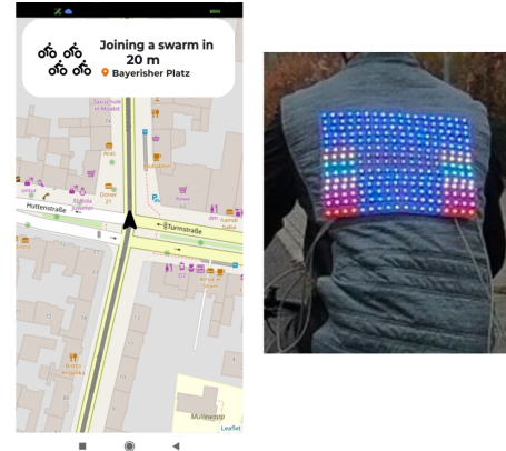
Fig. 3. Left: Show a notification on the smartphone when bicyclist joins a swarm. Right: Signalling on the LED matrix when a cyclist is joining the swarm (which has more than 15 members)
