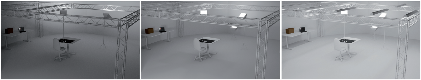
Figure 4: Illustrations of the laboratory setup in our three lighting conditions Dark, Medium and Bright (left to right). Studio lamps and lamps on the ceiling were used to adjust the environmental illuminance.
