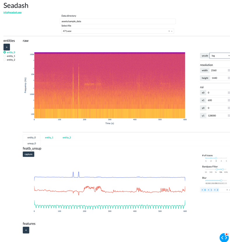
Figure 2. A screenshot of the Seadash application. Its main user interface (UI) elements are a file input element (top), a list of entities (left), and the data visualisation panels (centre-right, taking the largest part of the UI area). These are split between a spectrogram (top) and designed features (bottom). Each feature is a sub-tab of an entity.
