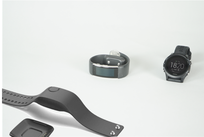
Figure 7.5: Empatica E4, Microsoft Band v2, and Garmin Forerunner 935 used for skin-based CL measures 57 .
