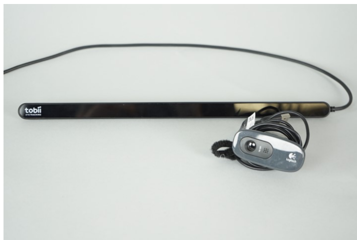
Figure 7.3: A Logitech webcam and the Tobii 4C eye tracker for eye-based CL measures.
