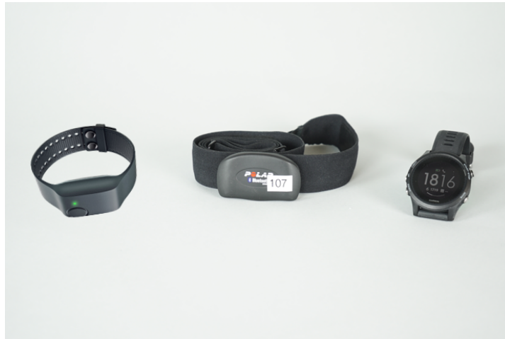
Figure 7.4: The Empatica E4, Polar H7 and Garmin Forerunner 935 for heart-based CL measures 56 .
