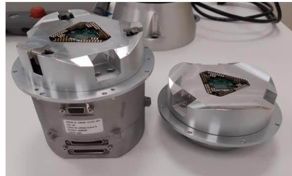
Figure 9 – Active SIROM (left), Passive SIROM (right). PERIOD benchmarking versions
