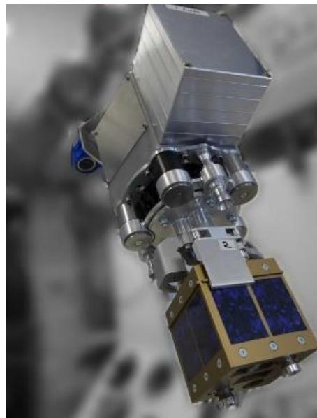
Figure 7 – The Multi-Purpose Tool with Cube Sat Gripper and a cube sat module
