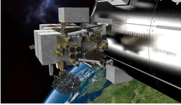
Figure 1 – The PERIOD Boxes mounted on the Bartolomeo platform outside of the Columbus module
