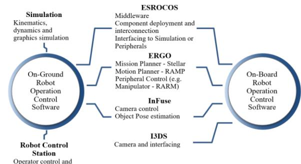
Figure 5 – Distribution of Software Components between Ground- and Space-Segment
