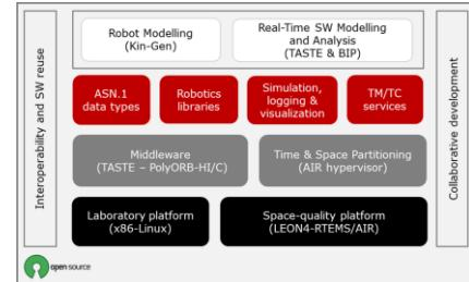
Figure 13 – The ESROCOOS software architecture
