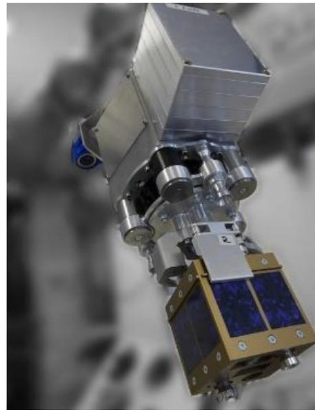
Figure 7 – The Multi-Purpose Tool with Cube Sat Gripper and a cube sat module
