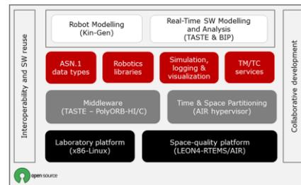
Figure 13 – The ESROCOS software architecture
