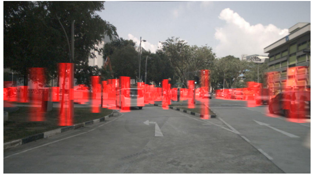
Figure 1. Visualization of the camera image, augmented with the uncertainty weighted RCS channel values highlighted in red.
