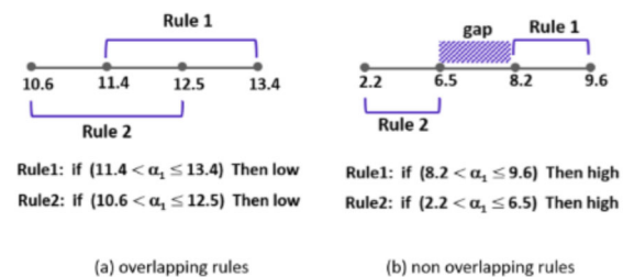
FIGURE 4. Rules sets with single term each rule sharing similar features and classes. In example (a) there is an overlap between rules and in example (b) the rules do not overlap.
