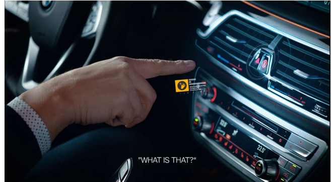
Figure 1: Driver makes a pointing gesture to interact with the car. Image courtesy of [1]
