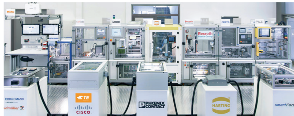
Figure 3: The SmartFactory KL pilot plant for Industrie 4.0 meets the three goal criteria "Mechantronic Changeability", "individualized mass productions" and "internal and cross-company networking". Image source: © C. Arnoldi
