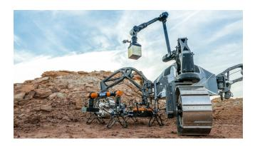
Figure 2: Multi-Robot Scenario: SherpaTT is handing over a sample container to Coyote III for return to the lander. Coyote III has the modular manipulation arm SIMA attached which is currently in a pose to facilitate the container hand-over.
