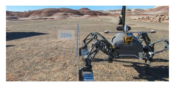
Figure 14: Experiment setup in Flat-Terrain. The DGPS module is connected to SherpaTT's rear EMI.
