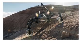
(b) SherpaTT in the steepest section of the slope with active roll-pitch adaption.
