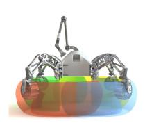
(b) Overlapping workspaces as seen from side. Rover model shown in standard Cross-Stance configuration.
