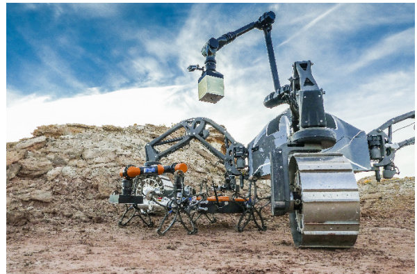
Fig. 14. Payload exchange between SherpaTT and Coyote III in the context of the TransTerra multi-robot system
