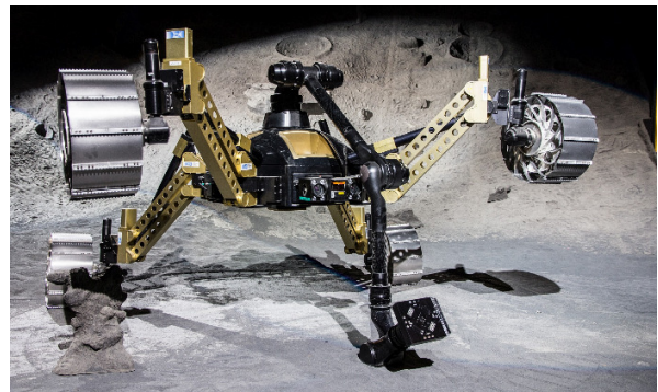
Fig. 11. Sherpa using its manipulator to lift front wheels off the ground (credit: DFKI GmbH)
