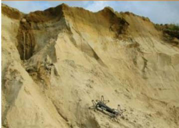
(Fig. 1) The Asguard robot climbs a loose sandwall with 40 degree incline
