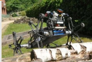
(Fig. 2) The Asguard v3 system uses its on board sensors and computing capabilities to autonomously navigate through difficult terrains
