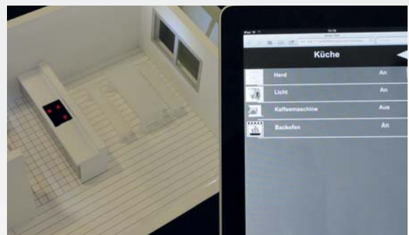
Interactive control of the miniature home via tablet computer or smartphone
